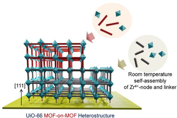
Scheme 1 Schematic illustration of UiO-66 MOF-on-MOF epitaxial, oriented heterostructure formation, using a room temperature self-assembly approach (solid bars = linkers and octahedron =  $Zr^{4+}$  node).
