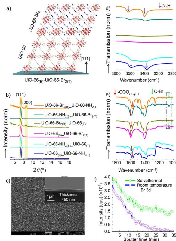
Fig. 3 (a) Illustration of a MOF-on-MOF geometry for UiO-66(B)-UiO-66-Br<sub>2(T)</sub>, (b) out-of-plane XRD patterns of the heterostructures, (c) SEM morphology and cross-section images of UiO-66(B)-UiO-66-Br<sub>2(T)</sub>, (d and e) IRRAS spectra of the heterostructures showing the specific intensity changes for -N-H, -C-Br and asymmetric -COO vibrations, and (f) -Br (3d) signal at different sputtering times for UiO-66(B)-UiO-66-Br<sub>2(T)</sub> and UiO-66(B)-UiO-66-Br<sub>2(T)/solvo</sub>.
