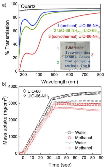
Fig. 2 (a) Transmission spectra (at 298 K) of bare quartz, the UiO-66-NH<sub>2</sub> thin films synthesized under the new ambient conditions and by the solvothermal method and UiO-66-NH<sub>2(B)</sub>-UiO-66(T) grown on quartz substrates, inset: optical images of the thin films; (b) water and methanol vapour uptake profiles of the UiO-66 and UiO-66-NH<sub>2</sub> thin films at 298 K.
