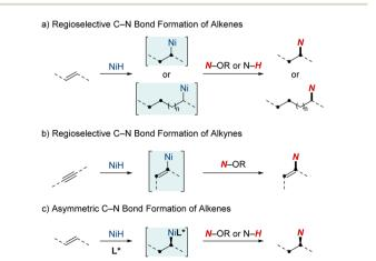
Scheme 1 NiH-catalyzed hydroamination and hydroamidation of alkenes and alkynes.
