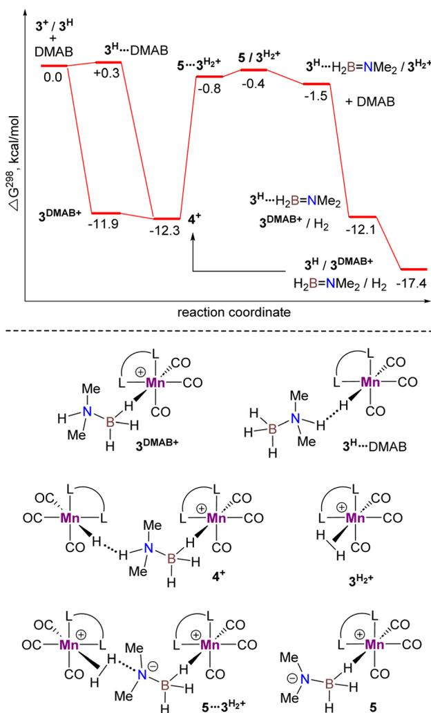
Fig. 5 Calculated Gibbs energy profile for DMAB dehydrogenation catalyzed by a  $3^+/3^H$  couple at the  $\omega$ B97XD/def2-TZVP level in toluene (dihydrogen bond interactions are indicated as dotted lines, non-interacting molecules are separated by a slash) and structures of the key intermediates (bottom).
