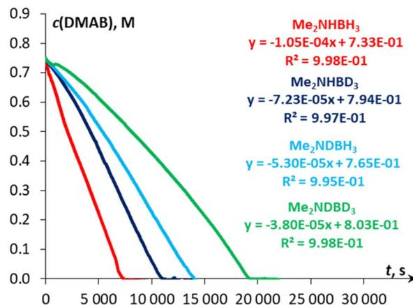
Fig. 4  $c(\text{DMAB})$  vs. time plots for the initial reaction rate determination of  $\text{Me}_2\text{NHBH}_3$ ,  $\text{Me}_2\text{NHBD}_3$ ,  $\text{Me}_2\text{NDBH}_3$  and  $\text{Me}_2\text{NDBD}_3$  ( $c_0 = 0.75 \text{ M}$ ) dehydrogenation catalyzed by  $3^{\text{Br}}$  (0.1 mol%) in the presence of  $\text{NaBPh}_4$  (1.0 mol%) in PhCl at 60 °C.
