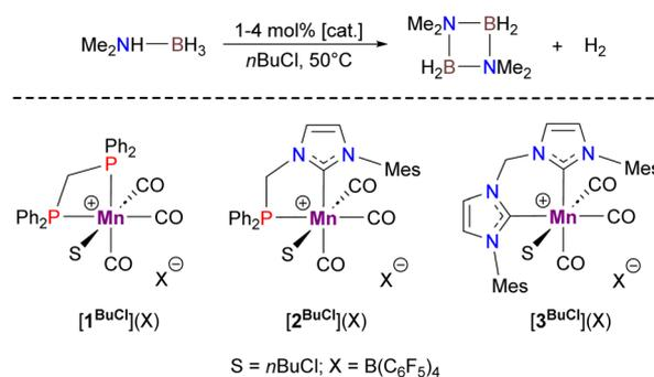
Scheme 2 DMAB dehydrogenation catalyzed by cationic Mn(I) complexes [1–3<sup>BuCl</sup>](B(C<sub>6</sub>F<sub>5</sub>)<sub>4</sub>).
