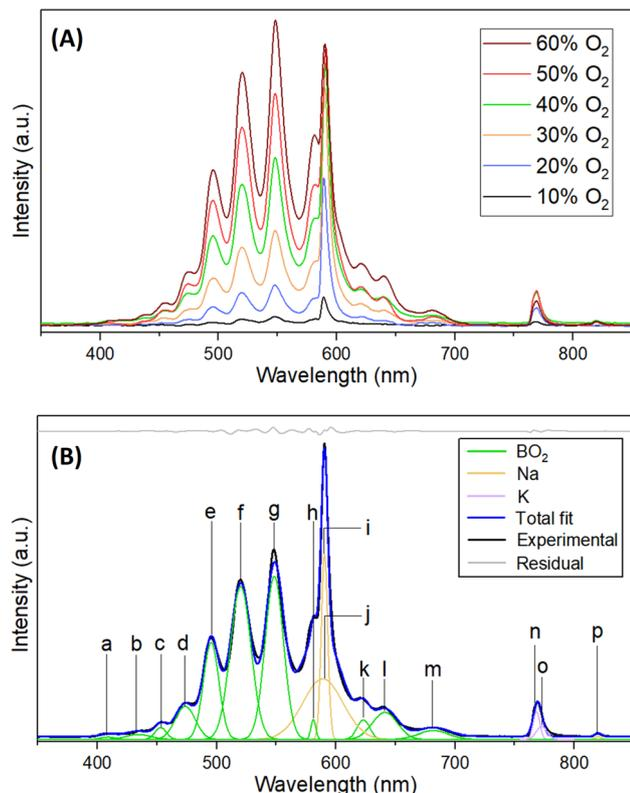
Fig. 3 (A) Stacked plot of the most intense spectra for the [EMIM][CBH]-WFNA ignition reactions at different molecular O<sub>2</sub> concentrations. (B) Deconvoluted flame emission spectrum upon ignition in 40% O<sub>2</sub>/60% Ar atmosphere at 10 ms since merging.
