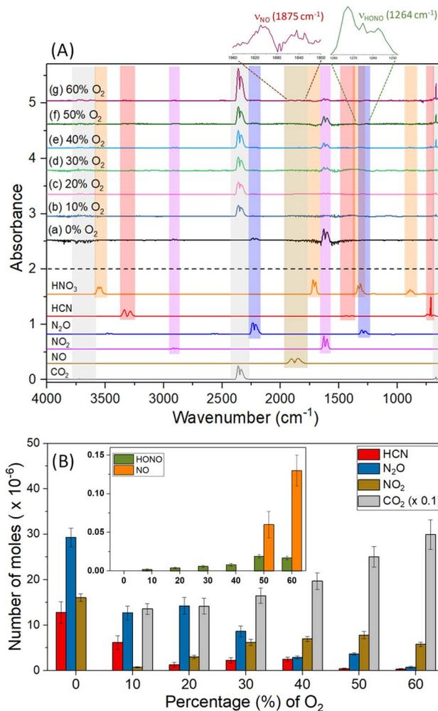
Fig. 4 (A) FTIR spectra and (B) quantification of gas-phase products formed in the [EMIM][CBH]-WFNA reactions as a function of molecular O<sub>2</sub> contents.
