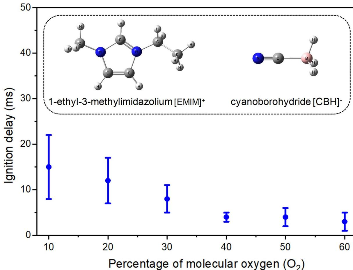
Fig. 1 Measured ignition delays (IDs) for the reaction of [EMIM][CBH] (inset) with WFNA as a function of molecular oxygen (O<sub>2</sub>) contents inside the levitator process chamber. The errors in the ignition delays represent the 1 –  $\sigma$  errors in the averaged time differentials between individual merging and ignition frames.
