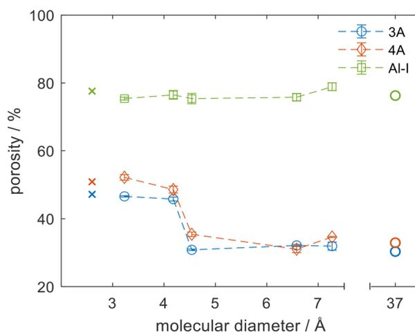
**Fig. 3** The porosity experienced by different probe molecules in alumina and zeolites 3A and 4A. The probe molecules are (left to right on the dashed line) water, methanol, *n*-decane, cyclohexane, and *o*-xylene. Helium pycnometry (x) and mercury porosimetry (o) results are shown for comparison.
