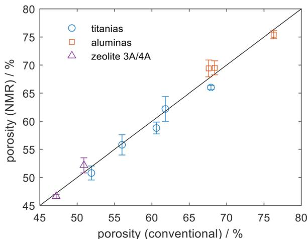
**Fig. 1** A comparison between the NMR porosity measurement and mercury porosimetry measurements applied to a range of titanias and aluminas. Skeletal densities of zeolites 3A and 4A were measured with helium pycnometry to ensure that the zeolite microporosity was captured. The solid line is a line of  $y = x$ . Errors bars represent the standard error of 3 measurements.
