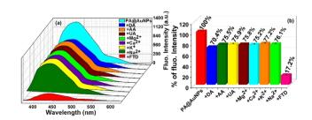
Fig. 1 (a) 3D diagram of fluorescence emission intensity changes of PA@AuNPs (1.0 mM) upon addition of various analytes (100  $\mu$ M) ( $\lambda_{ex}$  353 nm; slit width 5 nm), and (b) corresponding bar diagram shows the emission intensity of quenching percentage (STD = 3%).
