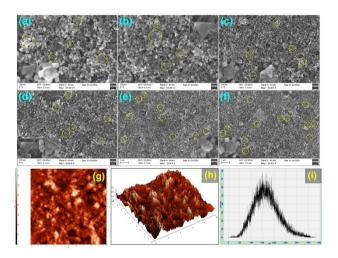
Fig. 6 (a-f) FESEM images of PA@AuNPs·FTD (a) 100 nm, (b) 100 nm, (c) 200 nm scale, (d) 200 nm, (e) 1  $\mu$ m, and (f) 1  $\mu$ m, respectively, and (g-i) AFM images of PA@AuNPs·FTD (g) 2D mode, (h) 3D mode, and (i) high profile graph. The FESEM and AFM images of PA@AuNPs can be found in Fig. SI11.‡
