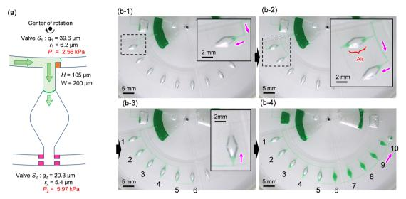
Fig. 2 Schematic representation of a method for outward sequential liquid dispensing into an array of 10 microchambers along the direction of centrifugal force. (a) Detailed design of the microchamber integrated with a pair of passive stop valves with different burst pressures. (b) Experimental results showing liquid dispensing into the microchambers at a rotational speed of  $1500 \text{ min}^{-1}$ .
