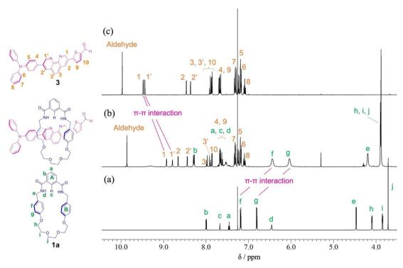
Fig. 1 Partial <sup>1</sup>H NMR spectra (400 MHz, CDCl<sub>3</sub>) of (a) macrocycle 1a, (b) pseudo[2] rotaxane, and (c) thread precursor 3.
