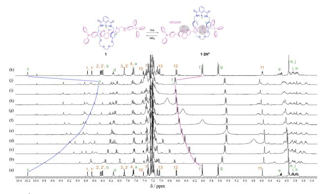
Fig. 3 Partial  $^{1}H$  NMR spectra (400 MHz, CDCl<sub>3</sub>) of (a) rotaxane 1, (b)–(j) the mixture obtained after adding TFA (1, 2, 3, 4, 5, 6, 7, 8, and 9 eq. respectively) to rotaxane 1 solution, and (k) the mixture obtained after adding NEt<sub>3</sub> (9 eq.) to the mixture obtained by addition of TFA (9 eq.) to rotaxane 1.
