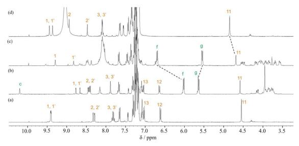
Fig. 4 Partial  $^1H$  NMR spectra (400 MHz, CDCl<sub>3</sub>) of (a) dumbbell 4, (b) rotaxane 1, (c) rotaxane  $1 \cdot 2H^+$  obtained after adding TFA (15 eq.) to rotaxane 1, and (d) dumbbell  $4 \cdot 2H^+$  obtained after adding TFA (15 eq.) to dumbbell 4.
