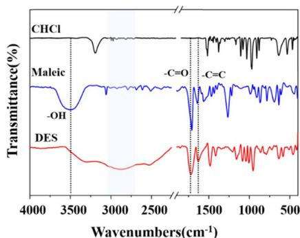
Fig. 1 FT-IR spectra of ChCl, maleic acid, and DES.
