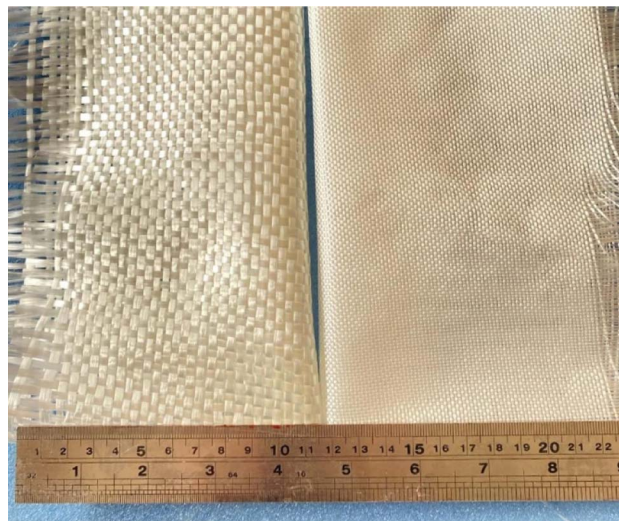
Fig. 1 300\text{ g m}^{-2} and 200\text{ g m}^{-2} glass fibers used in the study.
