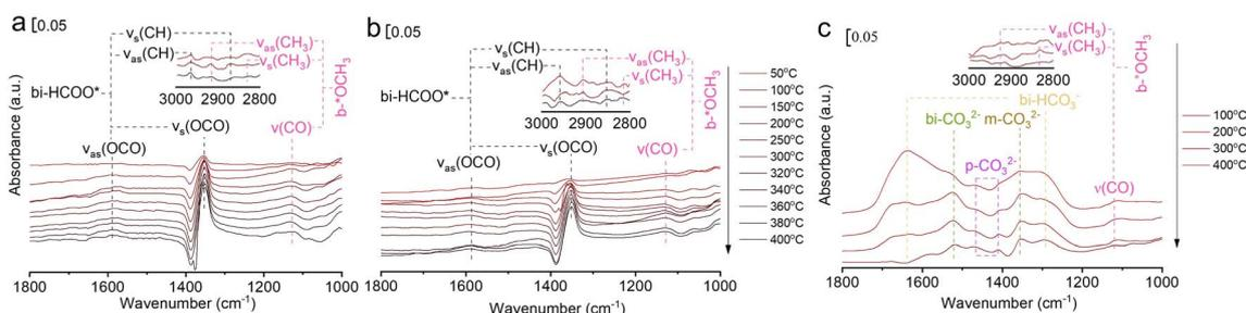
Fig. 3 *In situ* FTIR spectra of  $CO_2$  adsorption at different temperatures over (a)  $75In_2O_3-25ZrO_2$ , (b)  $In_2O_3$ , and (c)  $ZrO_2$ .
