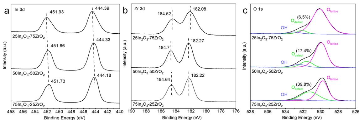
Fig. 1 XPS spectra of (a) In 3d, (b) Zr 3d, and (c) O 1s for the  $25\text{In}_2\text{O}_3$ - $75\text{ZrO}_2$ ,  $50\text{In}_2\text{O}_3$ - $50\text{ZrO}_2$  and  $75\text{In}_2\text{O}_3$ - $25\text{ZrO}_2$  catalyst.
