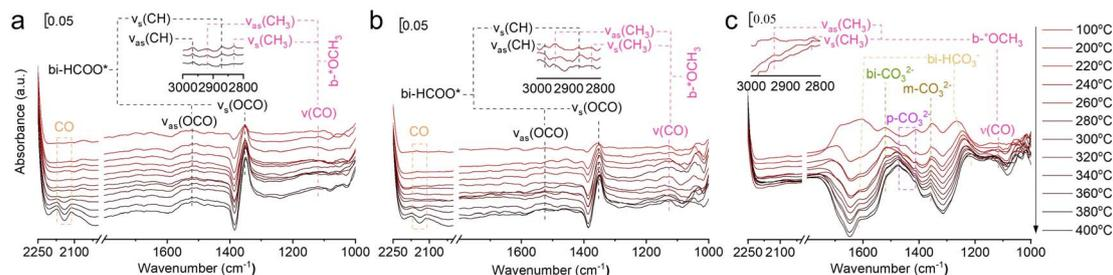
Fig. 4 *In situ* FTIR spectra of the reaction of CO<sub>2</sub> and H<sub>2</sub> over (a) 75In<sub>2</sub>O<sub>3</sub>-25ZrO<sub>2</sub>, (b) In<sub>2</sub>O<sub>3</sub>, and (c) ZrO<sub>2</sub>.
