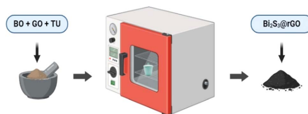
Fig. 1 Schematic of the one-pot solid-state synthesis process.
