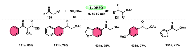
Scheme 80 I_2 -mediated direct \alpha -functionalization of ketones 113 .
