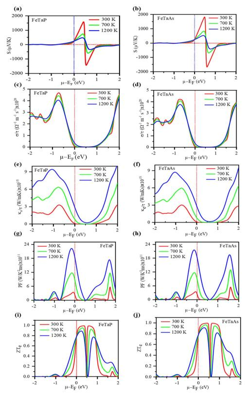
Fig. 9 The computed (a) and (b) Seebeck coefficients, (c) and (d) electrical conductivity, (e) and (f) electrical conductivities, (g) and (h) power factors, and (i) and (j) figures of merit (ZT) of FeTaP and FeTaAs as functions of chemical potential, respectively.
