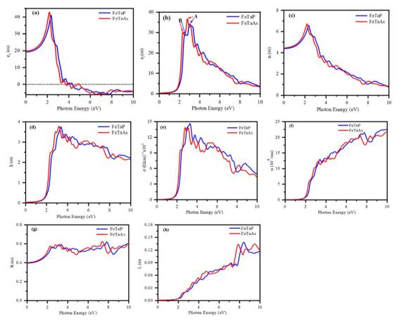
Fig. 7 DFT-calculated optical spectra of the (a) real component  $\varepsilon_1(\omega)$  and (b) imaginary component  $\varepsilon_2(\omega)$  of the dielectric function, (c) refractive index  $n(\omega)$ , (d) extinction coefficient  $k(\omega)$ , (e) optical conductivity  $\sigma(\omega)$ , (f) absorption coefficient  $\alpha(\omega)$ , (g) optical reflectivity  $R(\omega)$ , and (h) energy loss  $L(\omega)$  of FeTaX (X = P, As).
