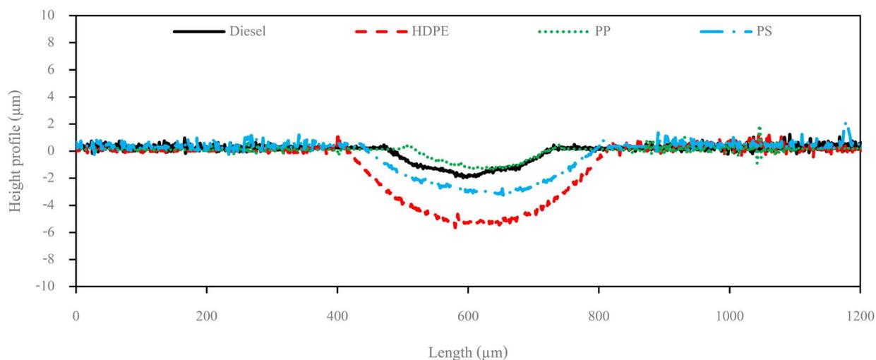
Fig. 13 Wear scar depth on HFRR lower specimen.
