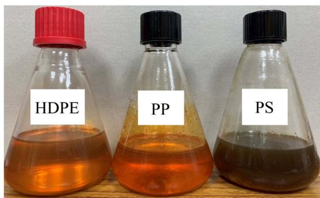
Fig. 4 Plastic pyrolysis oil after from the pyrolysis process.
