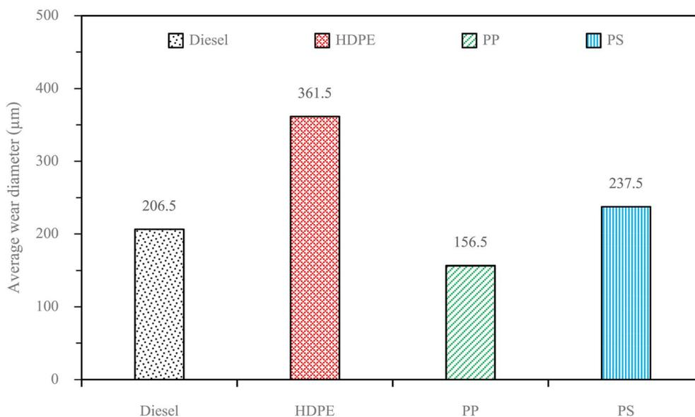
Fig. 10 Average wear scar diameters of test fuels.
