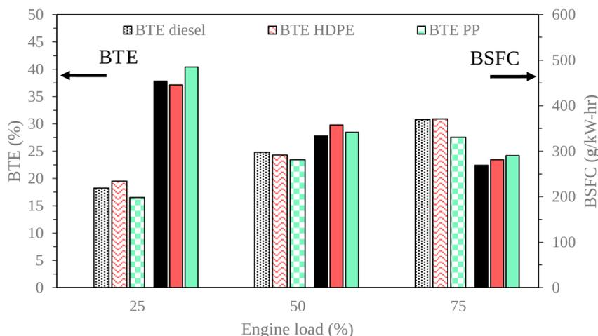
Fig. 15 Variation of brake thermal efficiency and brake specific fuel consumption with engine load.
