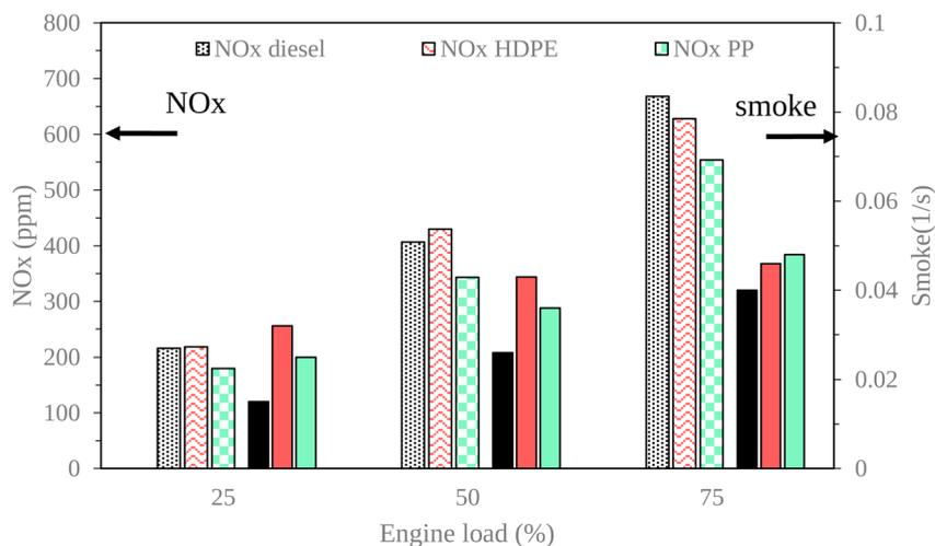
Fig. 19 Variation of NO<sub>x</sub> and smoke emission with engine load.
