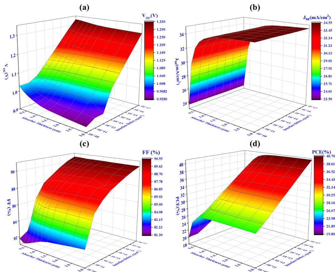
Fig. 7 Concurrent effect of PV performance factors (a)  $V_{\text{oc}}$  (b)  $J_{\text{sc}}$  (c) FF, and (d) PCE due to the alteration of interface (CIGS absorber/ $\text{Sb}_2\text{S}_3$  BSF) defect density.
