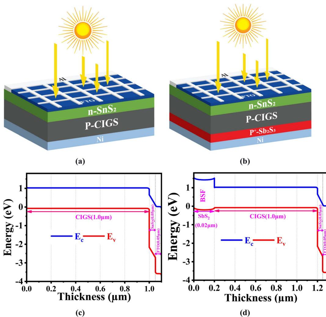
Fig. 1 The schematic structural design of suggested CIGS-based PV cell (a) without BSF, (b) with BSF, and the energy band diagram (c) without BSF, and (d) with BSF.
