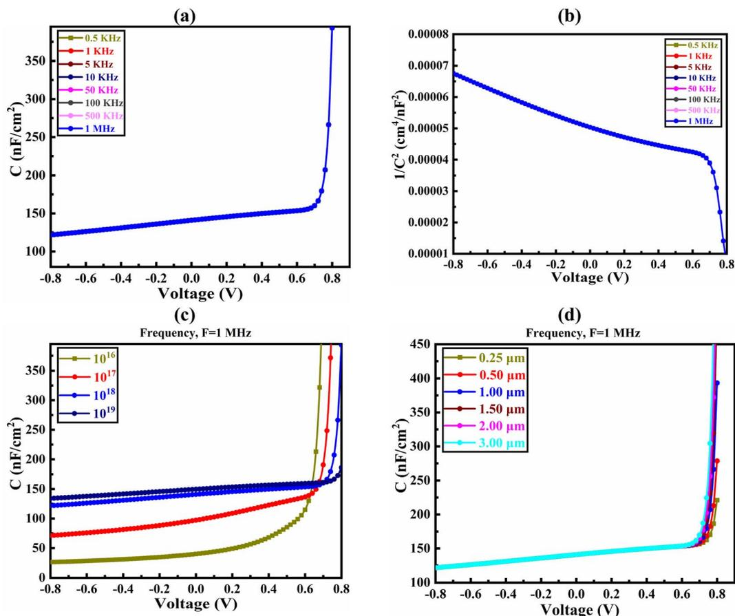
Fig. 5 Effect of  $C-V$  on the CIGS solar cell observed through with the (a) frequency variation, (b)  $1/C^2-V$  curve, (c) absorber doping variation, and (d) absorber thickness variation.
