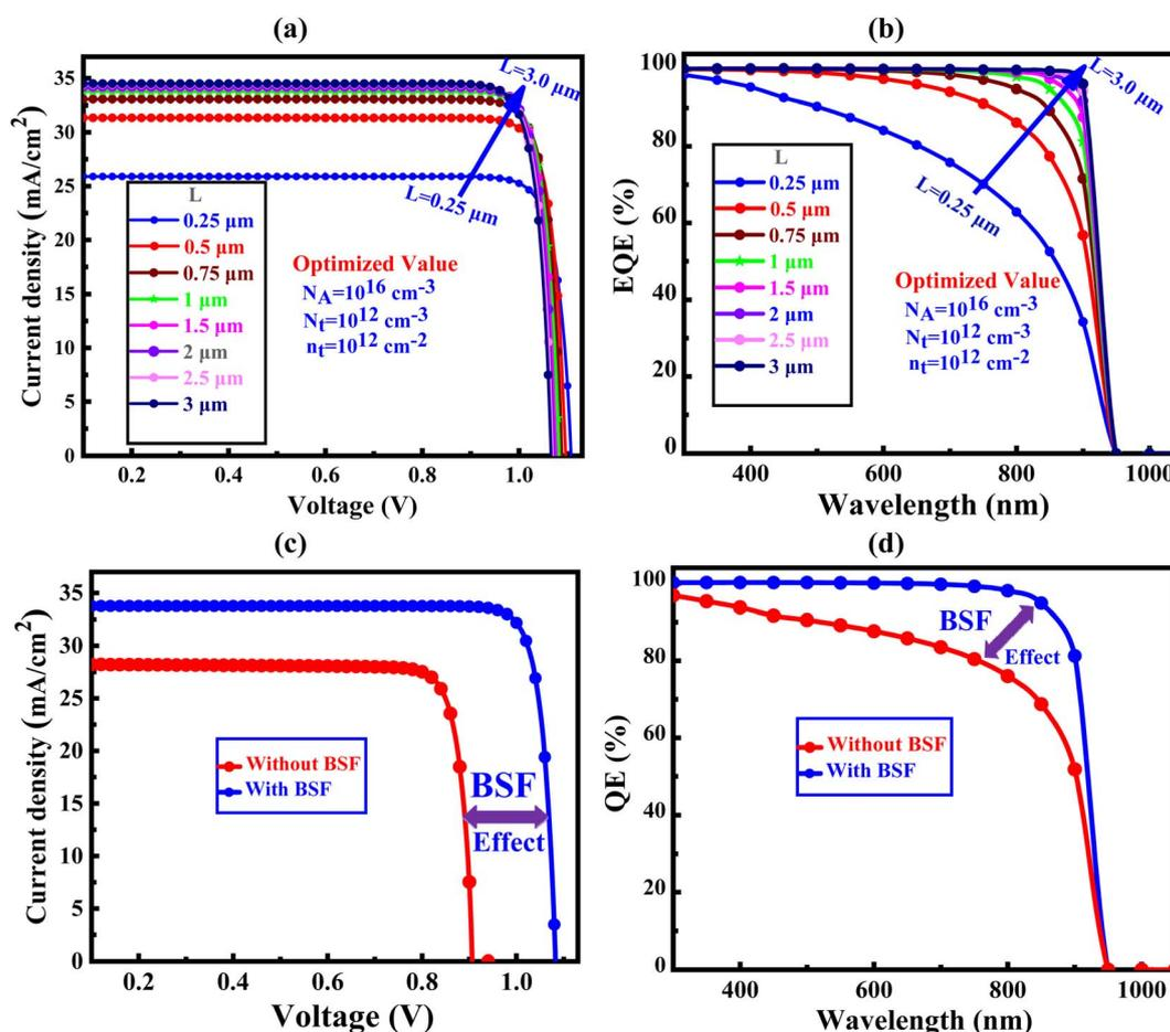
Fig. 9 Impact of absorber layer thickness with Sb<sub>2</sub>S<sub>3</sub> BSF layer on the (a)  $J$ - $V$ , and (b) QE, respectively and optimized value of proposed structure of (c)  $J$ - $V$  characteristics, and (d) QE curve comparison between with and without BSF.
