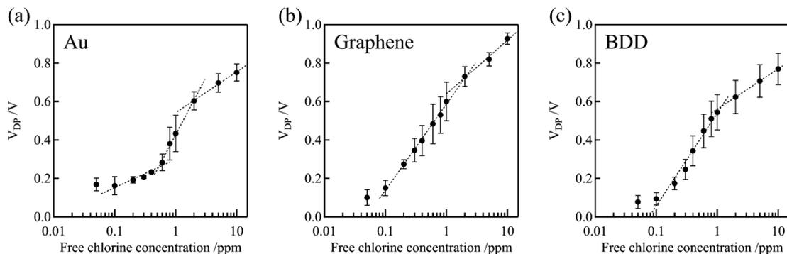
Fig. 7 Relationship between  $V_{DP}$  and free chlorine concentration for the Au, graphene, and BDD gate electrodes. The  $V_{DP}$  of the blank solution (0 ppm) for Au, graphene, and BDD gate electrodes were  $0.090 \pm 0.012$ ,  $0.12 \pm 0.032$ , and  $0.057 \pm 0.028$  V, respectively.
