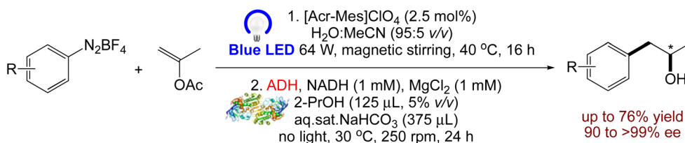
Scheme 10 Synthesis of enantiopure 1-arylpropane-2-ols from aryl diazonium salts via a photobiocatalytic cascade. 84
