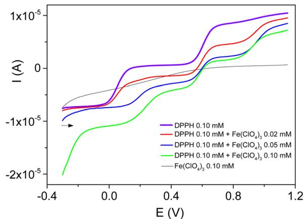
Fig. 3 Electrochemical signals at equilibrium recorded by linear sweep voltammetry at rotating glassy carbon electrode (900 rpm) at  $50 \text{ mV s}^{-1}$ , of DPPH 0.1 mM in TBAHFP 0.03 M acetonitrile solution, in presence of controlled amounts of  $\text{Fe}(\text{ClO}_4)_3$  (0 mM, 0.02 mM, 0.05 mM, and 0.10 mM).
