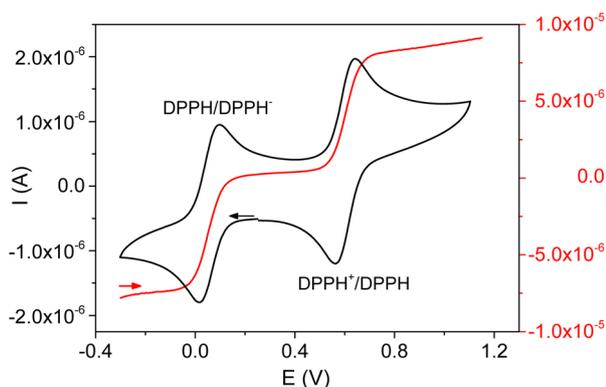
Fig. 2 Electrochemical signals of 0.1 mM DPPH in 0.03 M TBAHFP acetonitrile solution recorded using a glassy carbon electrode at  $50 \text{ mV s}^{-1}$ . Cyclic voltammogram at stationary electrode (black curve) and linear sweep voltammogram at rotating (900 rpm) electrode (red curve).
