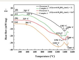
Fig. 10 DTA curves from 35 to 1500  $^{\circ}$ C for (a) Complex 1, (b) Precursor 4, (c) Complex 2, and (d) Precursor 5.
