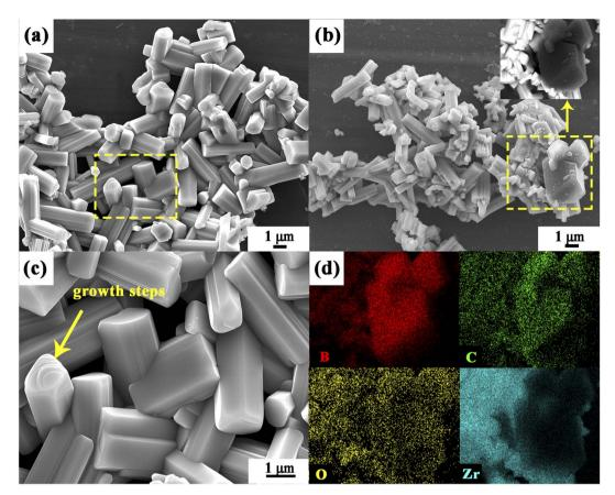
Fig. 16 Micrographs: SEM images of ZrB<sub>2</sub> powders prepared from (a) Precursor 4 and (b) Precursor 5 (the inset in (b) is the backscatter electron image); (c) enlarged image of the square in (a); (d) EDX elemental mappings of the polyhedral-like particles in the square of (b).
