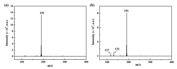
ESI mass spectra in the negative mode of (a) Complex 2 and (b) Complex 1.
