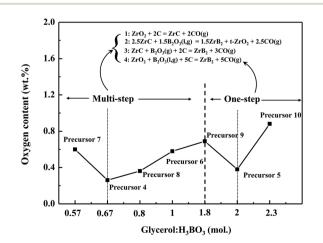
Fig. 14 Oxygen content of ZrB<sub>2</sub> powders prepared from Precursor 4 to Precursor 10 with different glycerol: H<sub>3</sub>BO<sub>3</sub> ratios (mol).
