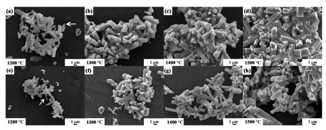
Fig. 17 SEM images of ceramic powders prepared from (a-d) Precursor 4 and (e-h) Precursor 5 after calcination for 1 h from 1200 to 1500 °C.
