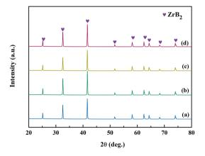
Fig. 13 XRD patterns of ZrB<sub>2</sub> powders obtained from (a) Precursor 7, (b) Precursor 8, (c) Precursor 9, and (d) Precursor 10.
