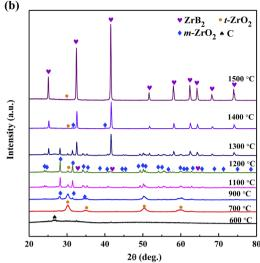
Fig. 11 XRD patterns of ceramic powders obtained from (a) Precursor 4 and (b) Precursor 5 after heating at different temperatures for 1 h.
