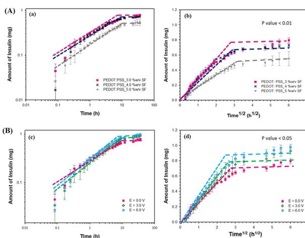
Fig. 7 Amounts of insulin released from insulin-loaded PEDOT:PSS/SF hydrogels under the effects of (A) SF concentrations and (B) electric voltages with PEDOT:PSS\_3.0% w/v SF. (a) and (c) Amounts versus time in the log–log plots, and (b) and (d) amounts versus time<sup>1/2</sup>.
