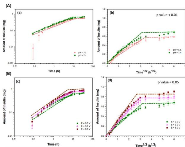
Fig. 8 Amounts of insulin release-permeation from insulin-loaded PEDOT:PSS\_3.0% w/v SF hydrogels under the effects of (A) pH values and (B) electric voltages. (a and c) Amounts versus time in the log-log plots, and (b and d) amounts versus time<sup>1/2</sup>.
