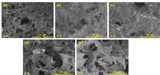
Fig. 5 Cross-section SEM images of PEDOT:PSS/SF hydrogels after swelling with and without electric voltages: (a) 3.0% w/v; (b) 4.0% w/v; (c) 5.0% w/v; (d) 3.0% w/v at  $E = 3.0$  V; and (e) 3.0% w/v at  $E = 6.0$  V.
