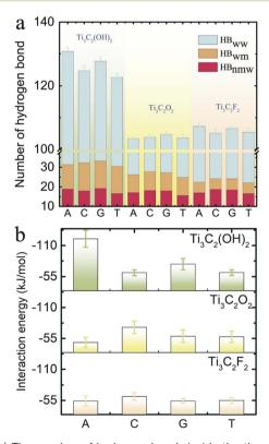
**Fig. 6** (a) The number of hydrogen bonds inside the three types of MXene nanopore, computed using the VMD plugin; the angle and distance cutoffs are 30° and 0.35 nm, respectively. (b) The interaction energy of ssDNA with the three types of MXene nanopore; this incorporates the Coulomb and Lennard-Jones energies. The error bars represent the standard deviation obtained from 15 independent runs.
