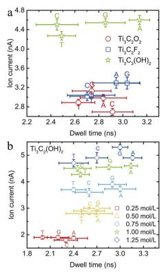
Fig. 4 (a) Ion current vs. dwell time for the three types of MXene nanopore. The green stars, red circles and blue squares represent the nanopores of  $Ti_3C_2(OH)_2$ ,  $Ti_3C_2O_2$  and  $Ti_3C_2F_2$ , respectively. (b) The ion currents and dwell times under different ion concentrations for the Ti<sub>3</sub>C<sub>2</sub>(OH)<sub>2</sub> nanopore.
