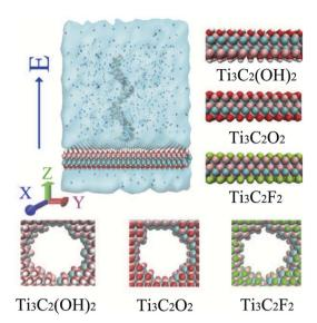
Fig. 1 The simulation model for ssDNA translocation through an MXene nanopore. For clarity, water molecules filling the simulation cell are not displayed. The right column shows the atomic structures of the three types of MXene membrane (mixed atom termination at the nanopore). The Ti, C, F, O and H atoms are depicted as pink, cyan, green, red and white spheres, respectively.
