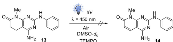
Scheme 4 Inhibition by TEMPO of the dehydrogenation of 13 to 14 .
