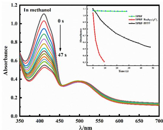
Fig. 2 The variation of absorbance of DPBF in methanol solution with the time of light exposure when PFPP is added as a photosensitizer (light: 460 nm,  $20 \text{ mW cm}^{-2}$ ); the inset is the plot of change in the absorption of DPBF at 415 nm versus time under light irradiation. (DPBF, DPBF + PFPP, DPBF +  $\text{Ru}(\text{bpy})_3\text{Cl}_2$ .)
