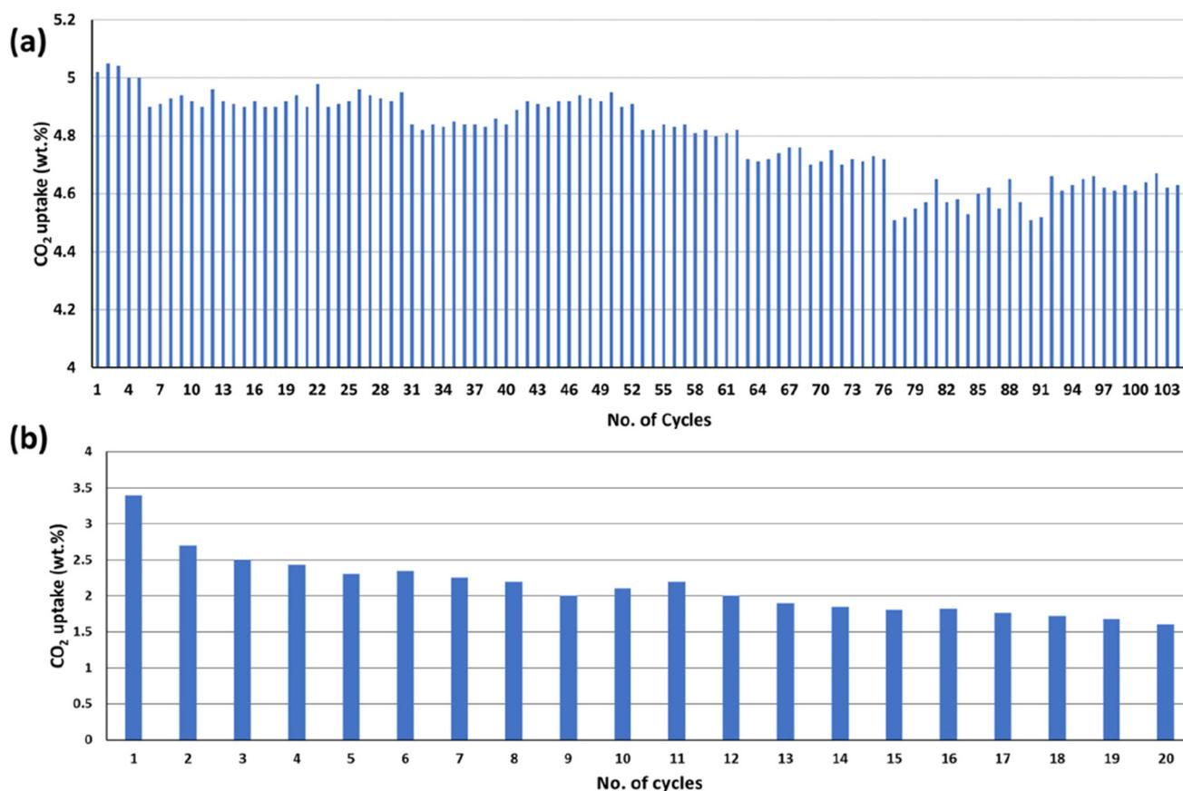
Fig. 8 (a) 105 adsorption-desorption cycles of silica-PEI bead. (b) 20 adsorption-desorption cycles of silica-HMDA bead. Adsorption was performed at 75 °C, a CO<sub>2</sub> flow rate of 25 mL min<sup>-1</sup> for 15 min, and desorption at 100 °C for 15 min under the flow of N<sub>2</sub> (50 mL min<sup>-1</sup>).
