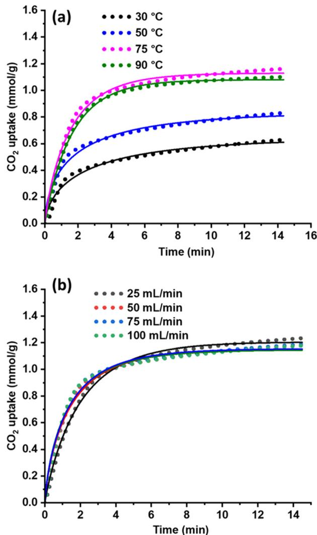
Fig. 6 Effect of adsorption temperature (a) and CO<sub>2</sub> flow rates (b) on CO<sub>2</sub> capture capacity and their corresponding Avrami model fitted curves of silica-PEI bead.
