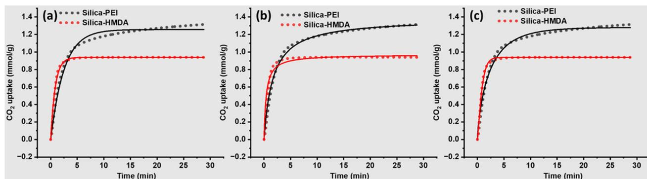
**Fig. 5** Fitting of CO<sub>2</sub> adsorption profiles using three kinetic models, (a) Pseudo first order kinetic model, (b) Pseudo second order, and (c) Avrami kinetic model.
