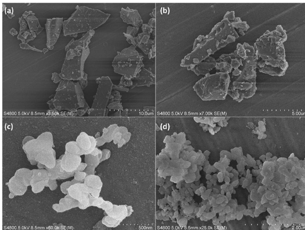
Fig. 3 SEM images of (a and b) BFS, (c and d) Silica.
