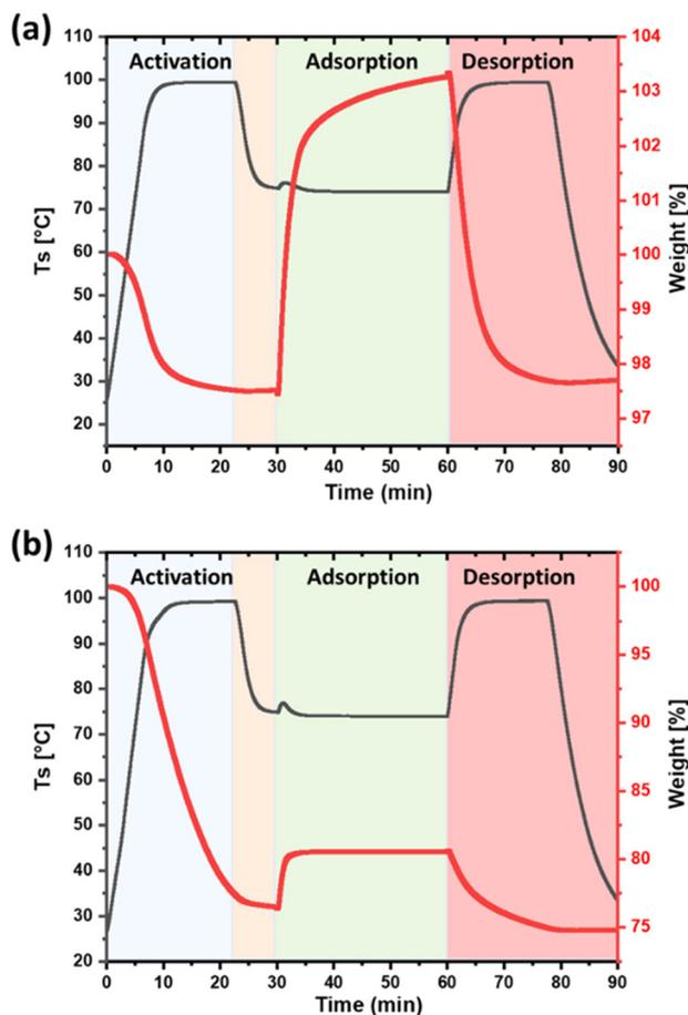
**Fig. 4** CO<sub>2</sub> adsorption on (a) silica-PEI bead and (b) silica-HMDA bead. Adsorption at 75 °C for 30 min, using 15% CO<sub>2</sub> in N<sub>2</sub>, desorption at 100 °C for 15 min.
