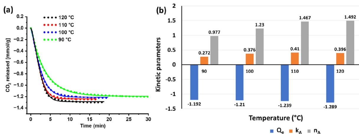
Fig. 7 (a) Desorption temperature optimization using Silica-PEI bead. (b) Kinetic parameters of four different desorption temperatures.
