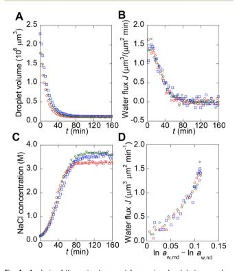
Fig. 4 Analysis of the water transport from microdroplets to nanodroplets during spontaneous emulsification. (A) Time course of the microdroplet volume, (B) water flux (J), and (C) NaCl concentration in the microdroplets. (D) Dependence of J on  $\ln a_{\rm w,md} - \ln a_{\rm w,nd}$ . Different symbols indicate different droplets in the same experiment. The NaCl concentrations of the pretreatment and initial microdroplet were 3 M and 0.2 M, respectively.
