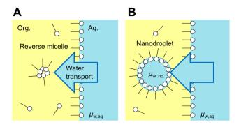
Fig. 1 Spontaneous emulsification induced by Span 80. Water transport to the reverse micelle of Span 80 in organic phase (A) and a nanodroplet is formed (B). The water transport continue until chemical potential of water nanodroplet  $(\mu_{w,nd})$  becomes equal to that in the aqueous phase  $(\mu_{w,aq}).^{23}$
