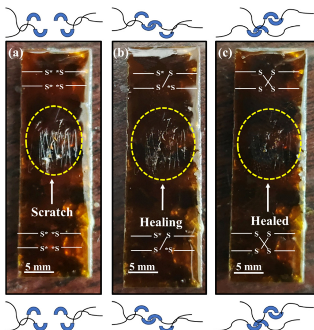
Fig. 6 Digital images of (a) scratched composite and healed composites after (b) 10 min and (c) 20 min.
