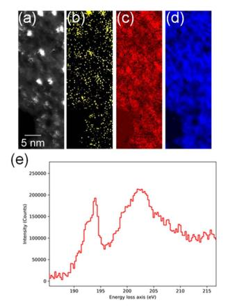
Fig. 2 (a) High-angle annular dark-field (HAADF)-STEM image showing Au nanocrystals, (b) EELS S-L<sub>2,3</sub> map (165.5-189.3 eV), (c) EELS B-K map (186.5-213.3 eV), (d) EELS C-K map (280.5-336.8 eV), (e) EELS data showing the fine spectral features for boron within the sulfur-doped boronic graphitic surfaces.
