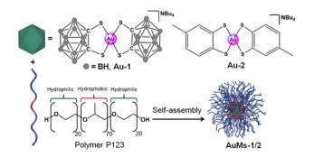
Scheme 1 Synthesis of AuMs-1 and AuMs-2 by self-assembly of block copolymer (P123) micelles containing encapsulated 16e Au(III) [Au(1,2-dicarba-closo-dodecarborane-1,2-dithiolato)<sub>2</sub>]  $[NBu_4]$  (Au-1) or  $[Au(4-methyl-1,2-benzenedithiolato)_2][NBu_4]$  (Au-2).
