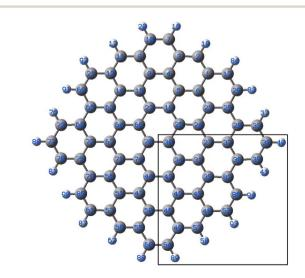
Fig. 4 Model graphene surface fragment 1 used for the DFT modelling. The atoms C27, C30-C36, C42-C43, C46, C48-49-49 and C82 were substituted with a B atom for each model.
