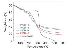
Fig. 2 Thermogravimetric curves of  $\gamma$ -CD and CD-MOFs. CD-MOFs were prepared by wash-free mechanochemical synthesis with different K+/CD ratios using KHCO3.
