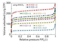
Fig. 3 N<sub>2</sub> adsorption/desorption isotherms of CD-MOFs prepared by wash-free mechanochemical synthesis. Before the measurements, the samples were degassed at 50 °C under vacuum for 6 h.
