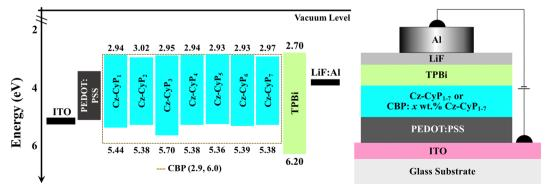
Fig. 5 Energy level diagram and schematic of the device architectures of solution-processed OLEDs.
