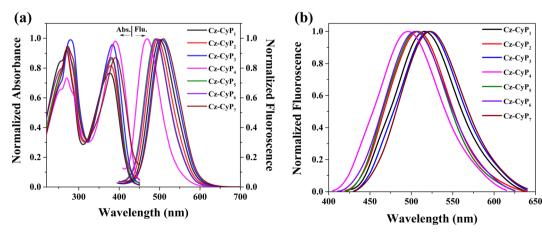
Fig. 2 (a) Absorbance spectra, (b) fluorescence spectra in solution and (c) fluorescence spectra in the thin film state of Cz-CyP<sub>1-7</sub>.
