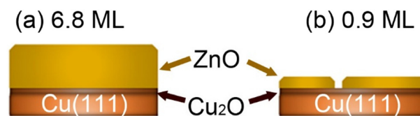
Fig. 1 Schematic illustration of the two ZnO/Cu(111) surfaces investigated herein as a function of the ZnO thickness. (a) 6.8 ML, (b) 0.9 ML.
