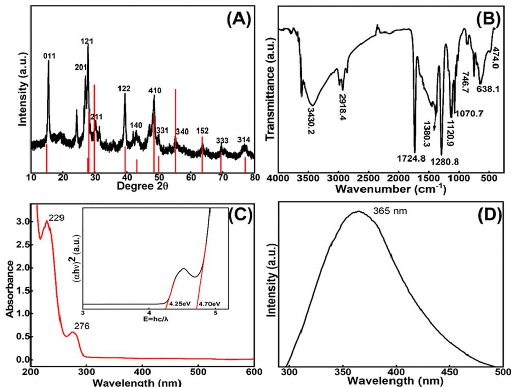
Fig. 2 (A) X-ray diffraction crystallography of  $\text{LaMn}_2\text{O}_5$ , (B) FT-IR spectra of rare phase nanostructure  $\text{LaMn}_2\text{O}_5$ , (C) UV-visible spectra of  $\text{LaMn}_2\text{O}_5$  (inset: the Touc plot of the UV graph representing the binding energy of  $\text{LaMn}_2\text{O}_5$ ) and (D) Photoluminescence spectra of rare phase nanostructure  $\text{LaMn}_2\text{O}_5$ .
