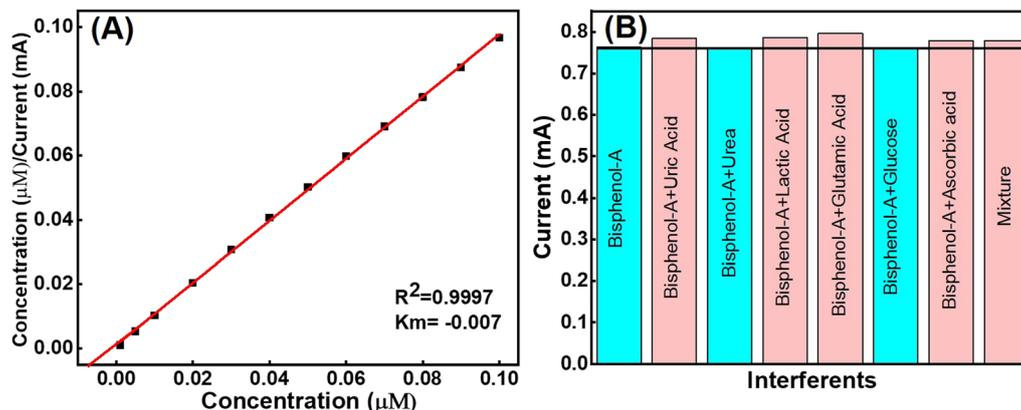
Fig. 8 (A) The Michaelis–Menten constant ( $K_m$ ) determined from the plot of concentration/current vs. concentration obtained from the sensing study and (B) the selectivity analysis for BPA using various interference analytes.
