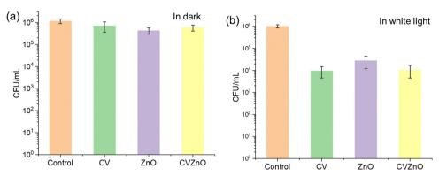
Fig. 5 Bactericidal activities of control, CV-dyed sample (CV), sample with ZnO NPs (ZnO), and CV-dyed sample with ZnO NPs (CVZnO) against E. coli in (a) dark and in (b) white light. The samples were exposed to white light source with an intensity of 512 lux for 4 h and another set was incubated for 4 h in dark room. All experiments were performed at 20 °C.
