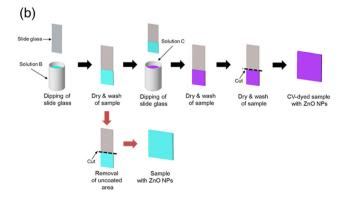
Fig. 1 Preparation of (a) control, CV-dyed sample, (b) sample with ZnO NPs, and CV-dyed sample with ZnO NPs. Solution A is a mixture of acrylic latex and toluene, solution B is a mixture of ZnO NPs and acrylic latex and solution C is crystal violet solution.
