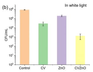
Fig. 4 Bactericidal activities of control, CV-dyed sample (CV), sample with ZnO NPs (ZnO), and CV-dyed sample with ZnO NPs (CVZnO) against S. aureus in (a) dark and in (b) white light. The samples were exposed to white light source with an intensity of 512 lux for 3 h and another set was incubated for 3 h in dark room. All experiments were performed at 20 °C.
