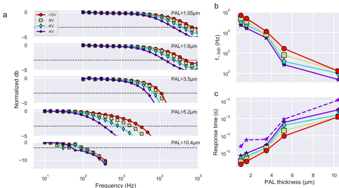
Fig. 5 a. Response time measured at various voltages for 1.05, 1.6, 3.5, 5.2, and 10.4  $\mu\text{m}$  PAL thickness; b bandwidth ( $f_{-3\text{dB}}$ ) and c. response time of the photodetector with various PAL thickness as obtained from the signal bandwidth measurements (dash line shows the response time measured by impedance fitting under a bias of -4 V).
