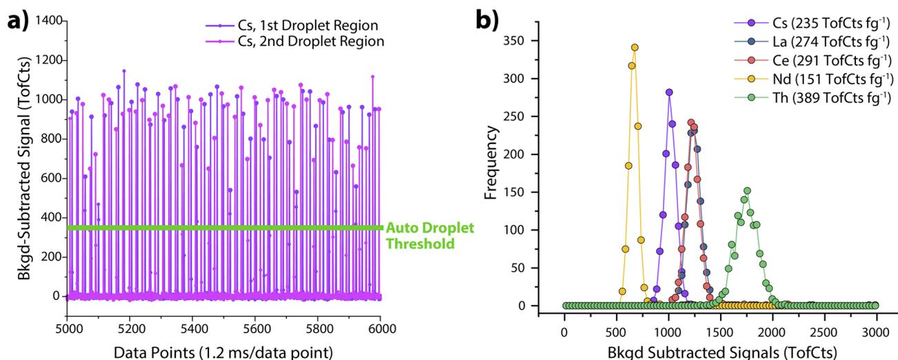
Fig. 4 (a) A small region (1000 data points, 1.2 s) of droplet signals from the plasma uptake standard, *i.e.* Cs. Droplets are typically introduced into the ICP at 40–50 Hz. (b) Histograms of analyte signals from the droplets are used to determine average absolute sensitivities (shown in parentheses in the legend). The droplets for this measurement were  $\sim 64 \mu\text{m}$  in diameter and the concentrations of all analyte elements were  $\sim 30 \text{ ng mL}^{-1}$ .
