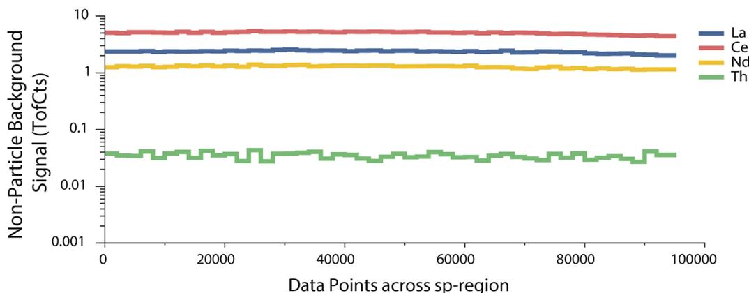
Fig. 3 Time-dependent average background signals ( $\lambda_{\text{bkgd}}$ ) for analyte elements are determined in the first step of TOF-SPI. These  $\lambda_{\text{bkgd}}$  values are based on iterative outlier analysis with  $L_C$  at  $\alpha = 0.001$  as the outlier boundary. Background value arrays are saved to the HDF5 file and used in step 3 of TOF-SPI for particle finding.
