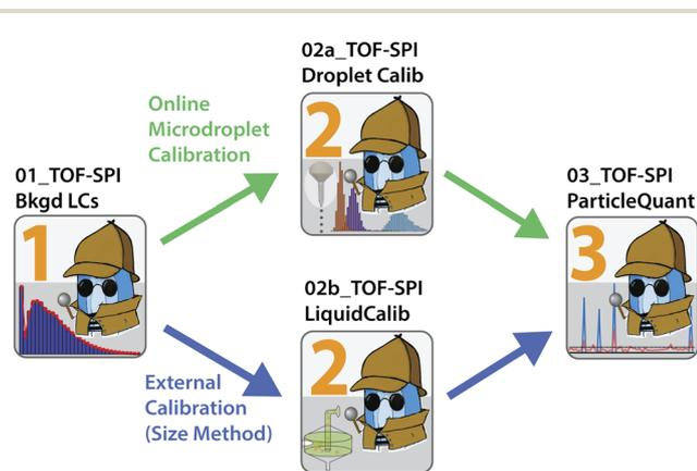
Fig. 1 General workflow of TOF-SPI programs for analysis of spICP-TOFMS data collected with calibration achieved with either online microdroplet calibration (top, green path) or external calibration *via* the particle-size method (bottom, blue path). Each spICP-TOFMS data file is processed in three steps—1, 2a, 3 or 1, 2b, 3—as indicated in the figure.
