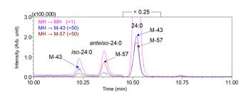
Fig. 8 Iso-24:0 is characterized by high [M-43]<sup>+</sup> (blue trace) in contrast to high [M-57]<sup>+</sup> (brown trace) in anteiso-24:0. Straight chain 24:0 has both ions at similar levels. Reprinted with permission from Wang et al.54 Copyright 2020 American Chemical Society.
