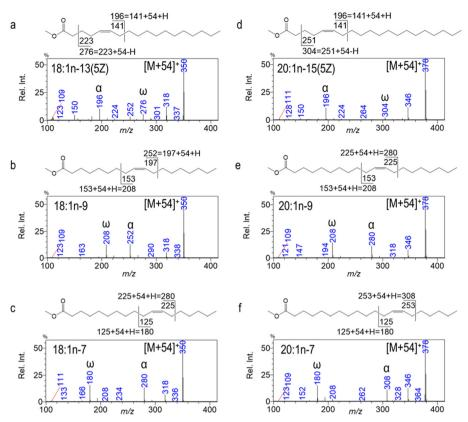
Fig. 2 CACI-MS/MS spectra of unusual  $\Delta 5$  18:1 and 20:1; all [M + 54]  $\rightarrow$  products. Reprinted with permission from Wang et al.<sup>23</sup> Copyright 2021 Elsevier Ltd.
