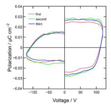
Fig. 6 P-V hysteresis curves of the MISIM ([ITO|PC|ET-PRBT|PC|Aq]) device at room temperature.
