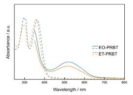
Fig. 2 UV-vis absorption spectra of the THF solution samples (broken curves;  $10^{-4}$  M) and thin films (solid curves; 30 nm) for ET-PRBT and EO-PRBT.
