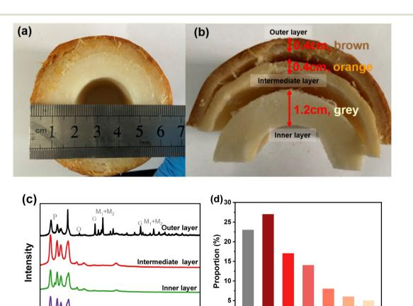
Fig. 1 (a) Cross-section photograph of the PCF, (b) photograph of different layers of the PCF, (c) XRD analysis of the used PCF and new PCF (G: goethite, Q: quartz, P: polypropylene,  $M_1$ : maghemite,  $M_2$ : magnetite), and (d) proportion of metal oxides in the PCF.
