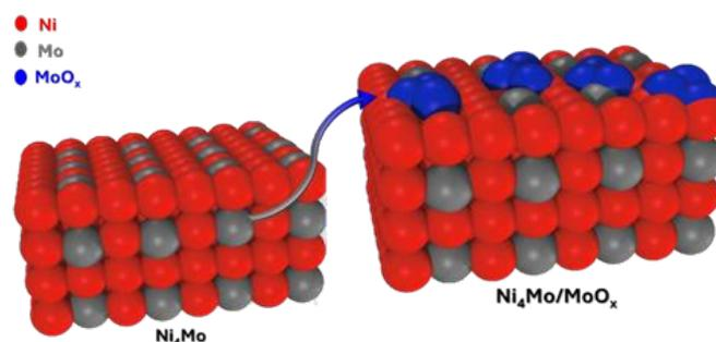
**Figure 8.** Schematic diagram of the surface re-organization of the catalyst during hydrogen evolution reaction
