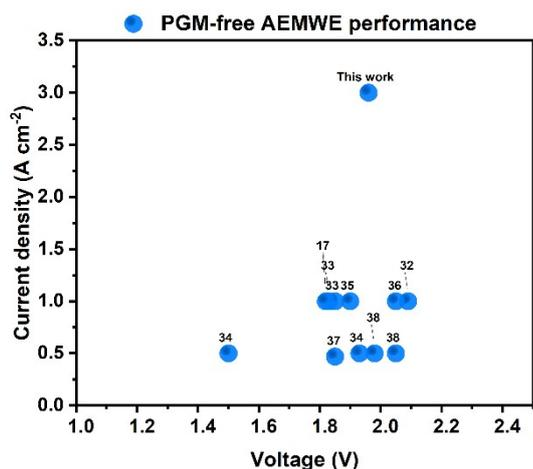
**Figure 9.** Comparison of the State-of-the-Art PGM-free AEMWE Cells. The numbers in the figure refer to the numbers of the references.
