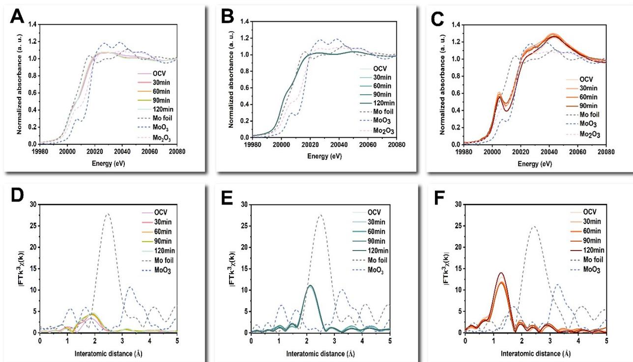
**Figure 7.** Operando XAS data : (A-C)-Mo K-edge XANES spectra of A- NiMo-AS1; B- NiMo-citric; C- NiMo-boric; (D-F)- Mo K-edge  $k^3$ -weighted EXAFS spectra for D-NiMo- AS1; E-NiMo-citric; F-NiMo-boric during activation in 1.0 M KOH.
