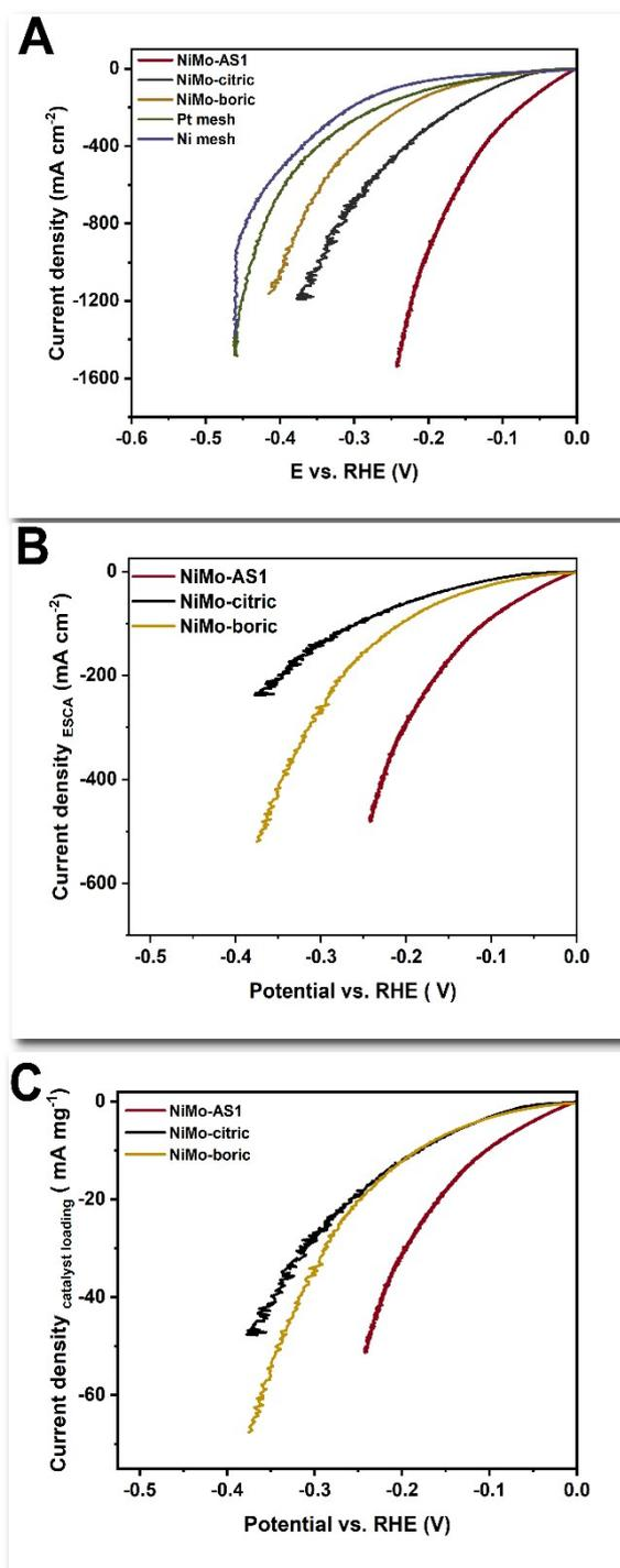
**Figure 1.** A. Linear sweep voltammetry (LSV) data showing geometric current densities of NiMo-AS1, NiMo-citric, NiMo-boric on Ni mesh support, bare Ni mesh, and Pt mesh; B. LSV data showing electrochemical active surface area (ESCA) averaged current densities of NiMo-AS1, NiMo-citric, NiMo-boric deposited on Ni mesh; C. LSV data showing catalyst loading averaged current densities of NiMo-AS1, NiMo-citric, NiMo-boric on Ni mesh.
