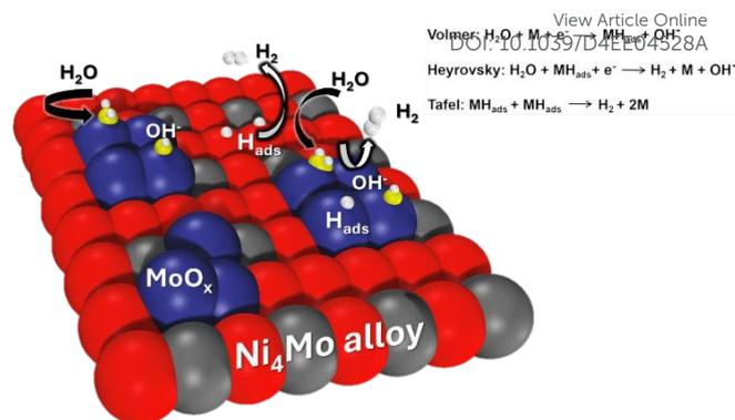
**Figure 10.** Schematic diagram of synergistic catalysis of alloy-oxide interface structures, in which the molybdenum oxide promotes water dissociation, and the alloy accelerates hydrogen combination.
