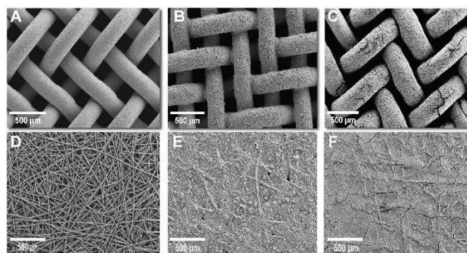
**Figure 4.** A. SEM image of bare Ni mesh; B. SEM image of the as-prepared NiMo-AS1 on Ni mesh; C. SEM image of the NiMo-AS1 on Ni mesh after HER at 1 A cm<sup>-2</sup>; D. SEM image of the bare C paper; E. SEM image of the as-prepared NiMo-AS1 on C paper; F. SEM image of the NiMo-AS1 on C paper after HER at 1 A cm<sup>-2</sup>.
