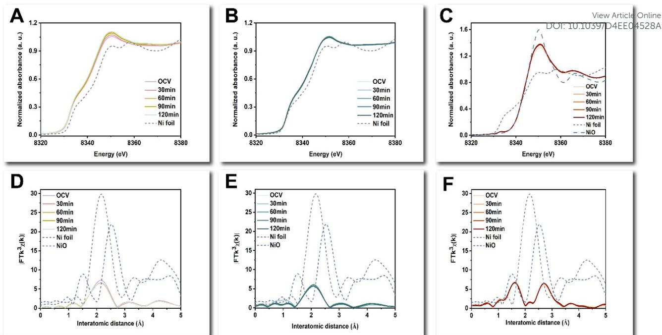
**Figure 6.** Operando XAS data : (A-C)-Ni K-edge XANES spectra of A- NiMo-AS1; B- NiMo-citric; C- NiMo-boric; (D-F)- Ni K-edge  $k^3$ -weighted EXAFS spectra for D-NiMo-AS1; E-NiMo-citric; F-NiMo-boric during activation in 1.0 M KOH.
