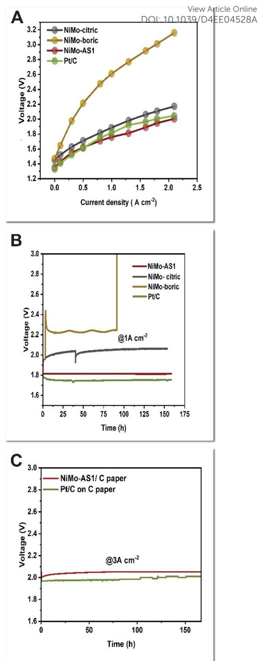
**Figure 3.** A. Polarization curves of AEMWEs with NiMo-AS1, NiMo-citric, and NiMo-boric on C paper as the cathode, respectively; B. Long-term electrolysis data at a constant current density of 1 A/cm<sup>2</sup> and cell temperature of 80°C; C. Electrolysis at a current density of 3 A/cm<sup>2</sup> at 80°C.
