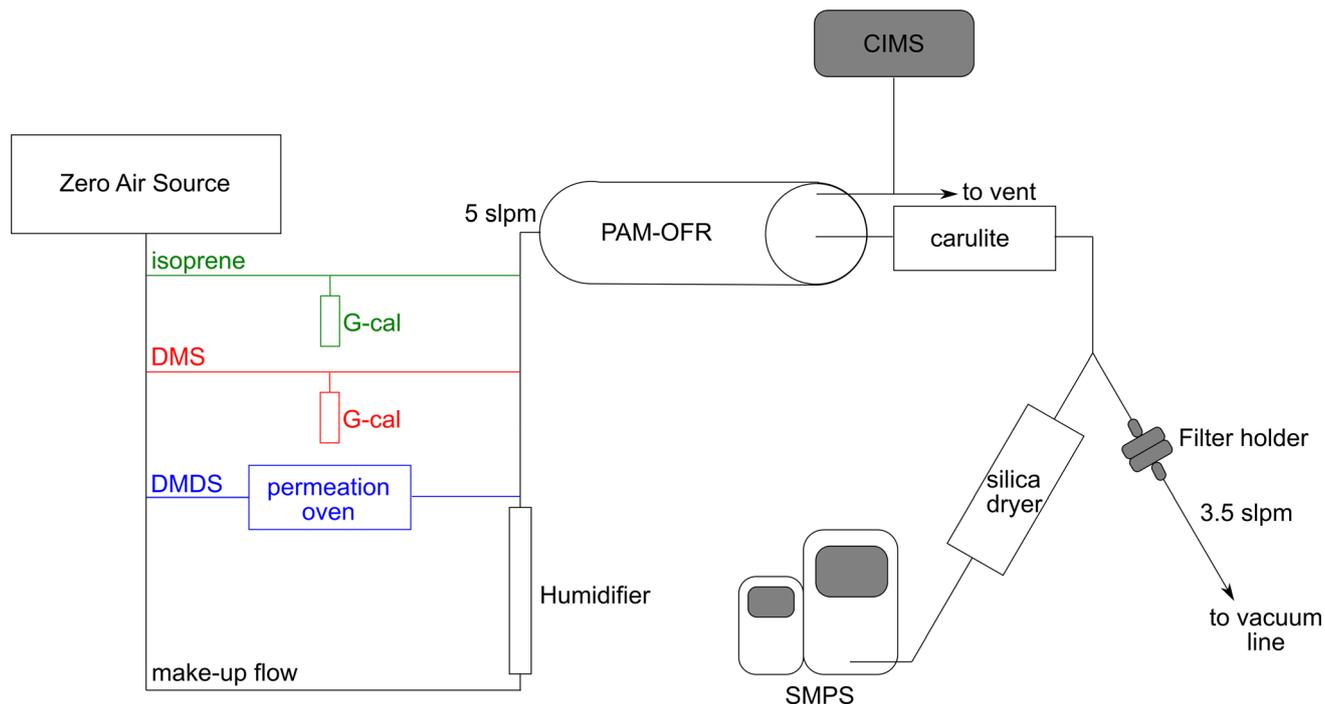
Fig. 1 Schematic diagram of experimental setup used for secondary marine aerosol reaction studies.
