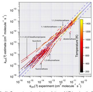
Fig. 11 Temperature-dependent predictions of k(T) based on the Estate technique, eqn (11), plotted against all available temperaturedependent measurements. With very few exceptions, it is noted that predictions become more accurate as temperature increases.
