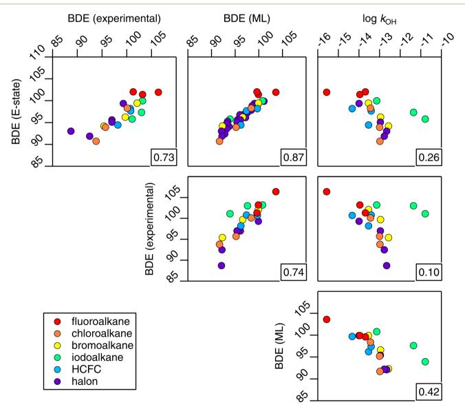
**Fig. 19** A correlation matrix of bond-dissociation energies estimated from E-state and machine-learning approaches, BDE(E-state) and BDE(ML) respectively, together with experimental BDE and  $k_{OH}$  data. The correlation coefficient for each relationship is provided in the bottom right corner of each panel.
