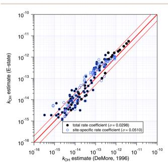
**Fig. 10** Estimates of  $k_{298}$  and site-specific  $k_i$  from the E-state technique compared with those of the DeMore group-additivity approach. As with the Atkinson approach, general better agreement is observed for total estimated rate coefficients compared with site-specific ones, as indicated by their respective standard errors ( $\sigma$ ) in parentheses.
