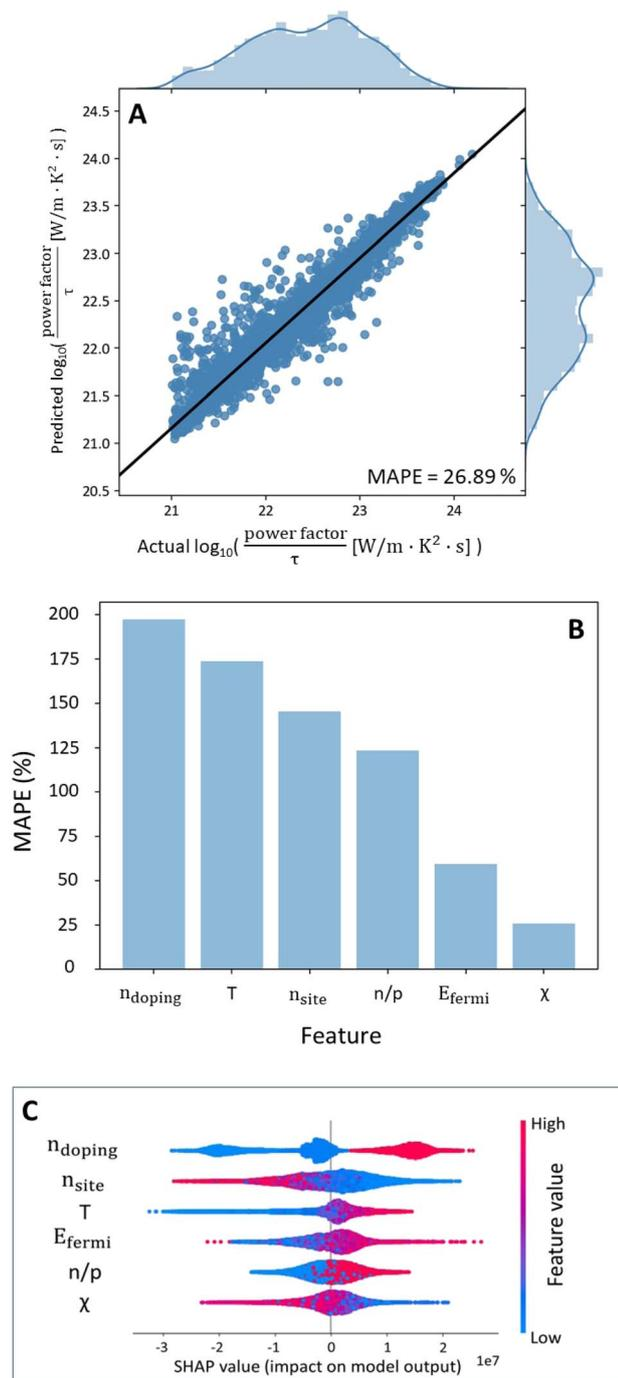
**Fig. 3** (A) Plot of prediction against actual  $\log_{10}(\text{power factor}/\tau)$  [W m<sup>-1</sup> K<sup>-2</sup> s<sup>-1</sup>] values for a random forest model trained on cubic structure materials with the 6 important features only. (B) Variation of error with feature addition to the random forest model. (C) SHAP feature importance (descending order of importance) for validating total gain feature importance.
