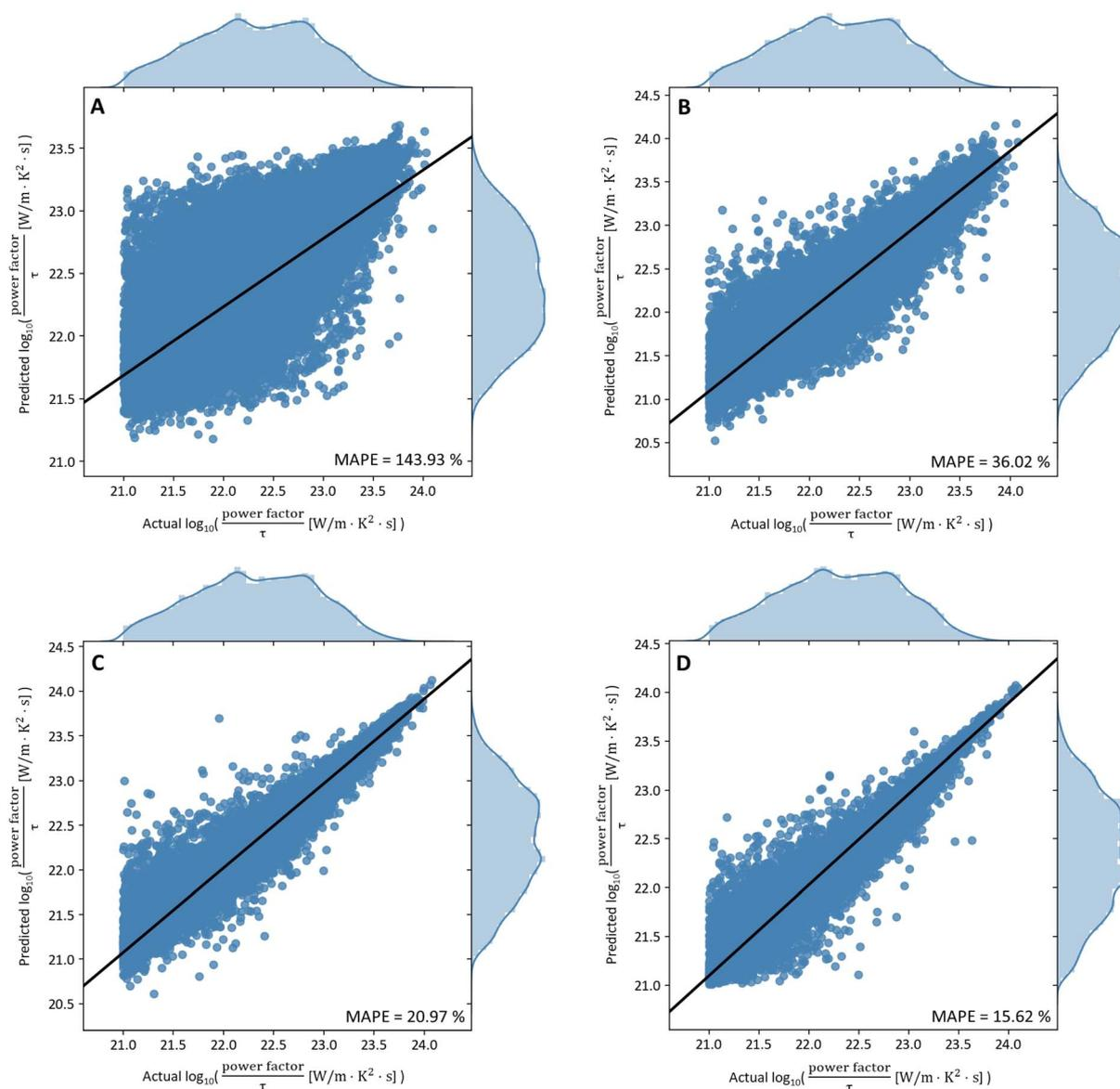
Fig. 1 Plots of prediction against actual  $\log_{10}(\text{PF}/\tau)$  [ $\text{W m}^{-1} \text{K}^{-2} \text{s}^{-1}$ ] values for different machine learning models. (A) CGCNN model. (B) DNN model. (C) XGB model. (D) RF model. The RF model shows the highest accuracy of 15.62% MAPE.
