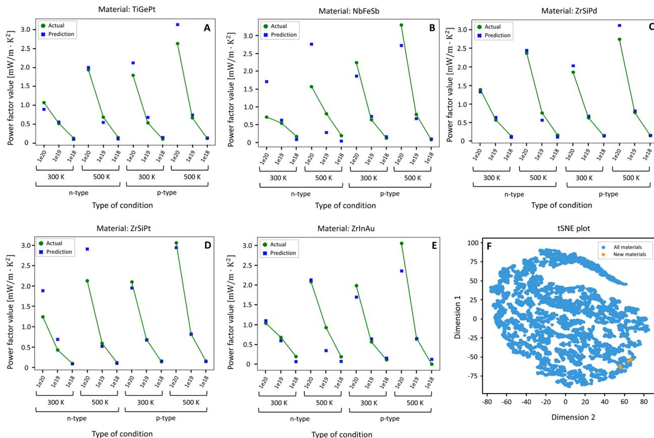
Fig. 5 Plots of predicted vs. actual (computed with DFT + BoltzTrap) power factor values [ $\text{mW m}^{-1} \text{K}^{-2}$ ] of the 12 chosen conditions of the 5 predicted thermoelectric materials and tSNE plot for comparing properties of the new materials with the materials in the training data. (A) TiGePt. (B) NbFeSb. (C) ZrSiPd. (D) ZrSiPt. (E) ZrInAu. (F) t-SNE plot.
