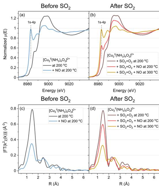
**Fig. 2** Cu K-edge XANES (a and b) and FT-EXAFS (c and d) spectra collected *in situ* during the exposure of the  $[\text{Cu}_2^{\text{II}}(\text{NH}_3)_4\text{O}_2]^{2+}$  species to NO at 200 °C (“not exposed to the  $\text{SO}_2$ ” protocol); exposure of  $[\text{Cu}_2^{\text{II}}(\text{NH}_3)_4\text{O}_2]^{2+}$  to  $\text{SO}_2 + \text{O}_2$ , then to NO at 200 °C, and at 300 °C (“exposed to the  $\text{SO}_2$ ” protocol).
