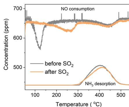
Fig. 1 Temperature-programmed reaction with NO, and  $\text{NH}_3$  desorption from  $[\text{Cu}_2^{\text{II}}(\text{NH}_3)_4\text{O}_2]^{2+}$  with (orange) and without (grey) prior exposure to  $\text{SO}_2$ .
