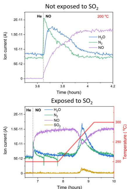
Fig. 4 Mass spectrometer data during exposure of the  $[\text{Cu}_2^{\text{II}}(\text{NH}_3)_4\text{O}_2]^{2+}$  complexes “not exposed to  $\text{SO}_2$ ” (top panel) and “exposed to  $\text{SO}_2$ ” (bottom panel) to NO. Masses:  $\text{H}_2\text{O}$ : 18, NO: 30,  $\text{N}_2$ : 28, and  $\text{SO}_2$ : 48.
