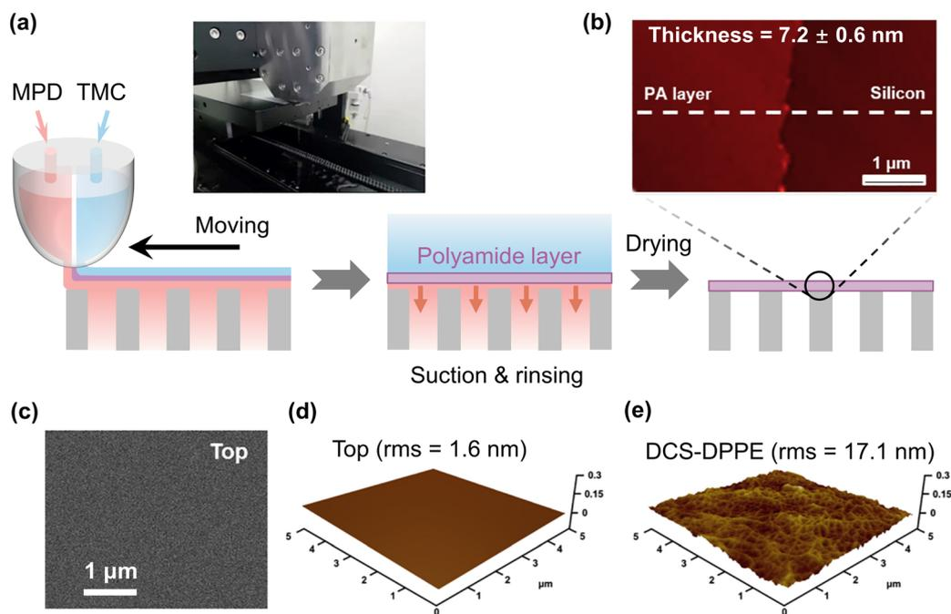
**Fig. 5** (a) Schematic view of the fabrication of polyamide membranes via the dual-layer slot coating method. (b) Cross-sectional AFM image of the polyamide layer on top of the silicon wafer surface. (c) SEM surface morphology, (d) AFM surface morphology, and (e) surface root-mean-square-roughness (rms) of the fabricated polyamide layer using the DSC method. Reproduced with permission from ref. 50, Copyright 2020, Elsevier B.V.
