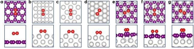
Fig. 4 Stable configurations of  $O_2$  adsorption on (a) graphene, (b) Pt(100), (c) Pt(110), (d) Pt(111), (e) Pt(100)@C, (f) Pt(110)@C, and (g) Pt(111)@C surfaces from top and side views. The red, purple, and grey balls represent O, C, and Pt atoms, respectively.
