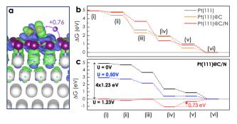
Fig. 8 (a) Charge transfers between O2 and the Pt(111)@C/N surface Color code: green: gaining electron region, blue: losing electron region (isosurface value of 0.002 e bohr<sup>-3</sup>). (b) Free energy profile of the ORR on the Pt(111), Pt(111)@C, and Pt(111)@C/N surfaces at  $U_{RHE} = 0$  V. (c) Free energy profile of the ORR on the Pt(111)@C/N surface at  $U_{RHE} = 0 \text{ V}$ (in black),  $U_{RHE}$  = 1.23 V (in red), and limiting potential  $U_L$  (in blue).
