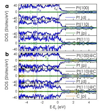
Fig. 3 Total DOSs and partial DOSs of (a) bare Pt and (b) Pt@C surfaces. The Fermi level ( $\varepsilon_{F_r}$  black dashed line) is found at 0 eV. Positions of the C pband center ( $\varepsilon_p$ , orange vertical line), Pt p-band center ( $\varepsilon_p$ , green vertical line), and Pt d-band center ( $\varepsilon_{d}$ , blue vertical line) are marked for comparison
