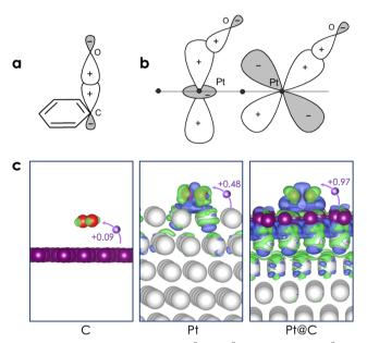
**Fig. 5** (a) Interaction between  $C(sp^3)-O(sp^3)$ , (b)  $Pt(d_{z^2})-O(sp^3)$  and  $Pt(d_{xz})-O(sp^3)$ . (c) Charge transfers between  $O_2$  and three surfaces: graphene, Pt(111), and Pt(111)@C. Color code: green: gaining electron region, blue: losing electron region (isosurface value of 0.002 e bohr $^{-3}$ ). The red, purple, and grey balls represent O, C, and Pt atoms, respectively.
