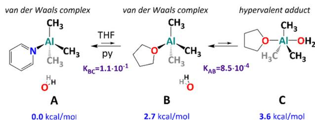
Fig. 4 Computationally modelled incipient complexes of AlMe<sub>3</sub> with H<sub>2</sub>O in the presence of neutral donor ligands.
