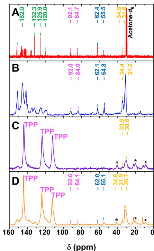
Fig. 3 The  $^{13}\text{C}$  NMR spectra of **1** in a  $\text{CS}_2$  solution with the internal standard of acetone- $d_6$  at 25 °C (A), of **1** in solid state (B), and the solid-state  $^{13}\text{C}$  CP MAS NMR spectra of 5%**1**@TPP- $d_{12}$  (C) and 10%**1**@TPP- $d_{12}$  (D). The black asterisks indicate spinning sidebands.
