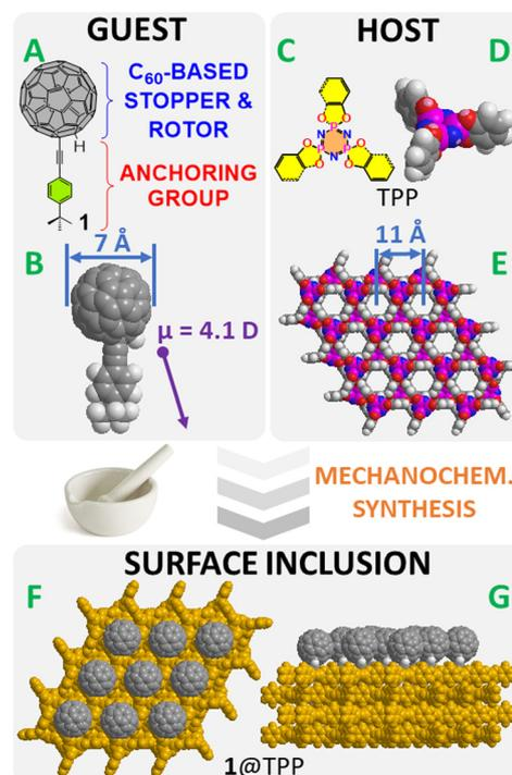
**Chart 1** The structure of the C<sub>60</sub> derivative **1** (A) and its space-filling model with a net dipole moment (B). The structure of the TPP molecule (C), the corresponding space-filling model (D) and a top view of a small fragment of hexagonal TPP (E). An idealized visualization of **1**@TPP: a top (F) and a side (G) view.
