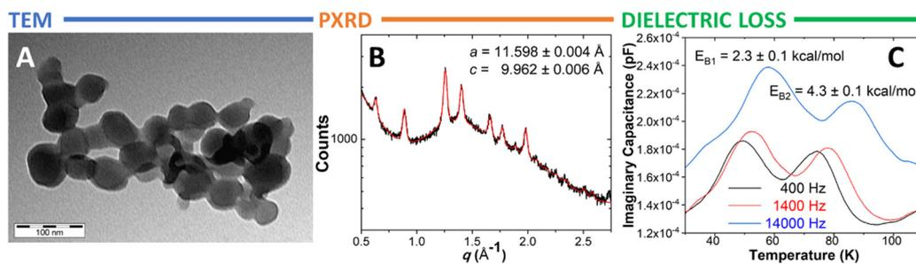
**Fig. 2** A TEM visualization of 10%**1**@TPP-*d*<sub>12</sub> (A). PXRD pattern of 10%**1**@TPP-*d*<sub>12</sub>. The black line represents the diffraction data, while the red curve reflects the fit (B). The dielectric loss of 10%**1**@TPP-*d*<sub>12</sub> recorded between 20 and 110 K. Black – 400 Hz, red – 1400 Hz, and blue – 14000 Hz (C).
