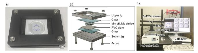
Fig. 2 Schematic of the microfluidic device mechanically clamped with a jig and the homemade time-lapse imaging equipment. (a) Photograph of the device clamped with a jig. (b) Configuration of the microfluidic device and the jig. (c) Photograph of the time-lapse imaging equipment.
