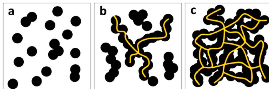
**Fig. 8** Schematic diagram showing the effect of filler loading and conductive network formation in carbon black composites, with (a) lower dosage, (b) medium, and (c) optimum loadings of carbon black depicting the percolation thresholds (reproduced with permission from ref. 140 (Copyright 2019, Springer Nature, licensed under a Creative Commons Attribution (CC BY) license)).
