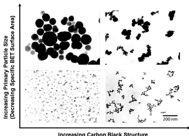
**Fig. 3** Morphological scheme showing the relationship between carbon black structure and primary particle size modified with permission from ref. 73 (Fig. 5, chapter 14, copyright 2017, Springer Nature, License number: 5360850466579).
