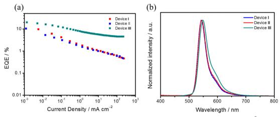
Fig. 6 (a) EQE versus current density curves of Devices I-III. (b) Electroluminescence spectra of Devices I-III at 500 cd m<sup>-2</sup>.
