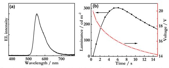
Fig. 7 (a) The steady-state EL spectrum. (b) The temporal evolution of the luminance (left y-axis, solid black squares) and the drive voltage (right y-axis, open red circles) for the ITO/PEDOT:PSS/26DCzPPy:POT2T: Sym-DiDiKTa:THABF<sub>4</sub>/Al LEC device. The LEC devices were driven by a constant current density of 77 mA cm<sup>-2</sup>.
