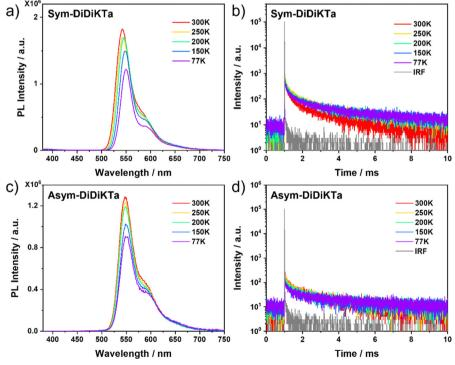
Fig. 5 (a and c) Temperature-dependent PL study of 1 wt% of Sym-DiDiKTa and Asym-DiDiKTa, respectively, in mCP,  $\lambda_{\text{exc}}$  = 350 nm. (b and d) Temperature-dependent time-resolved PL decays for 1 wt% **Sym-DiDiKTa** and **Asym-DiDiKTa**, respectively, in mCP matrix ( $\lambda_{\text{exc}} = 378 \text{ nm}$ ).
